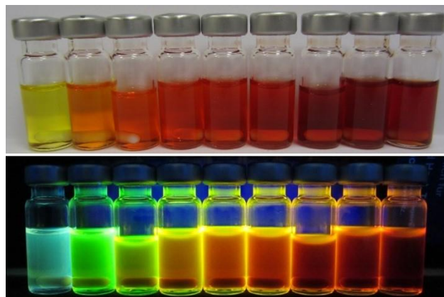
Fig. 1: Colloidal suspensions of CdSe quantum dots of increasing size from left (approximately 2.3 nm diameter) to right (approximately 4.0 nm diameter). Top: Samples viewed in ambient light vary in color from green–yellow to orange–red. Bottom: The same samples viewed under long-wave ultraviolet illumination vary in color from blue to orange–red.
