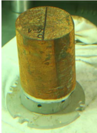
Fig. 3: Trepan sampled from the Greifswald Unit 1 RPV.
