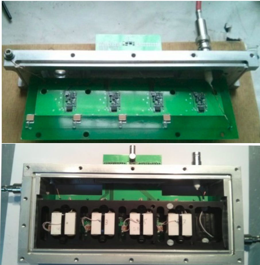
Figure 1. Top - The PCB readout board with HV distribution (HV capacitors) and preamplifier/shaper circuits fixed on the upper cover of the detector box; Bottom - RPCs of the prototype inside the box. On the photo four RPCs (white quadrat with black belt) are seen.
