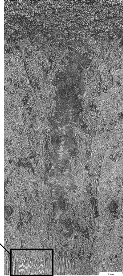
Figure 7: Channel-like segregation in the centre of a longitudinal section (same sample as Fig. 6)
