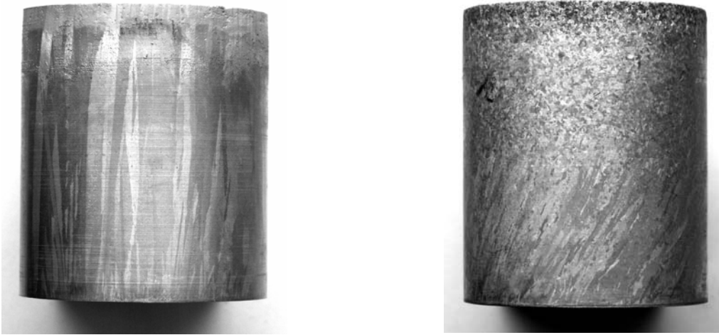
Fig. 5: Macrostructures visualized on the angular surface of the solidified samples: Ta = 0 (left) and Ta = 4.8 \cdot 10^6 (right)
