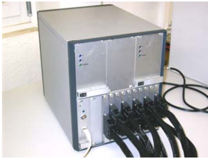
Fig. 2: Signal processing electronics (left) and view of one of the 10 pulse shaping and counting boards (right).
