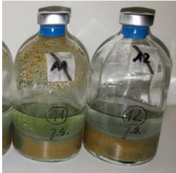
Figure 11: B36 microcosms containing supplemented Opalinus Clay pore water after 98 days incubation at 30 °C.
