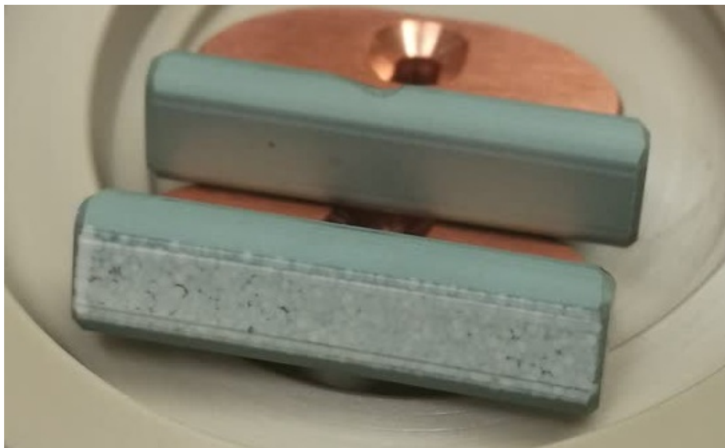
Figure 8.1: The picture of aged electrodes. The bottom electrode is anode, top electrode is cathode.
