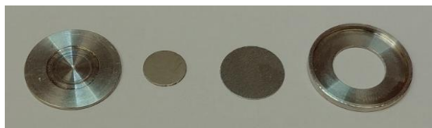
Fig. 2: Target capsule (from left to right: Al backing, Mg foil, Al foil, cover).
