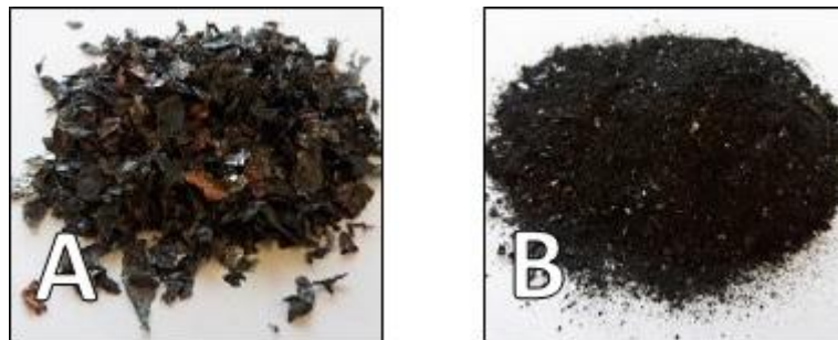
37 38 39 40 41 42 43 44 45 46 47 48 49 Figure 2 Pictures of representative samples of the LIB waste used in this study (A) overflow 50 and (B) underflow fractions
