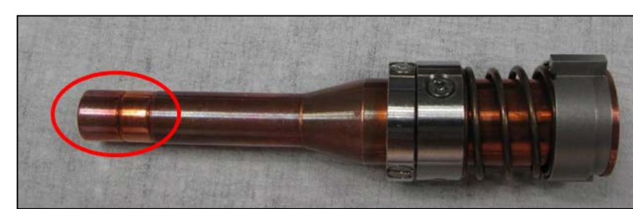
cathode (cathode body + plug)
