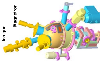
FIG. 1: Design study of the deposition chamber.
