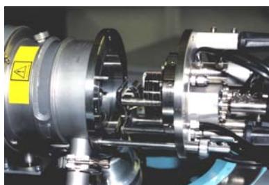
Commercial high temperature chamber (Otto) for annealing up to 2000°C in vertical scattering geometry.
