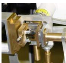
Commercial high temperature chamber (Otto) for annealing up to 2000°C in vertical scattering geometry.
