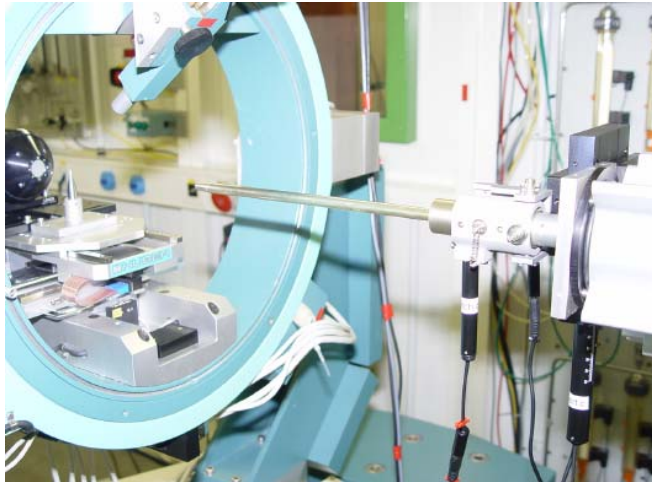
Fig. 3. Capillary inside the positioning system (pitch, roll, height, lateral movements) in front of the alignment setup at ROBL-MRH with CCD and calibration needle at center position of the 6-circle Huber goniometer.
