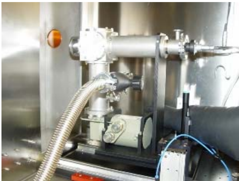
Fig. 1. The new cryostat mounted inside the glove box.
