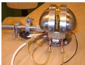
User designed annealing chamber for reactive gases .
