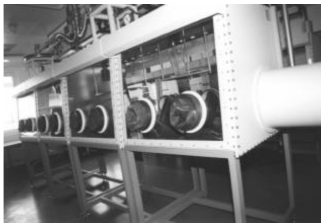
Fig. 3: View on alpha-glove boxes laser spectroscopy, UV-vis/FTIR-spectroscopy, photon correlation spectroscopy, field flow fractionation, equipment for electrochemical measurements, and ultra centrifugation. Modern equipment for \alpha -, \beta - and \gamma -spectrometry is also available.
