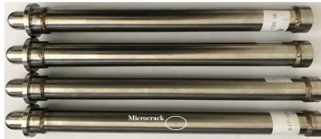
(a) Test section of heat transfer tubes with an axial micro-crack.
