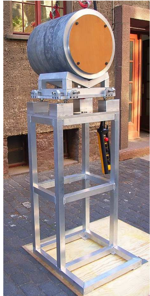
Fig. 3: Aluminium beam dump on its rack (test mounting).
