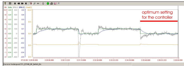
Fig. 5: Optimizing of the controller. (Green: Set Value with added step function).
