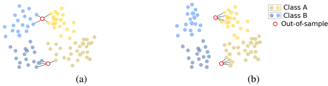
Fig. 2. Illustration of the limitation of the SNCA loss. (a) In the metric space produced by the SNCA loss, it will be challenging for KNN classifier to distinguish the out-of-sample images located near the border between the two classes. (b) By introducing CE loss, these two classes are further separated in the metric space, the same out-of-sample images in (a) can be accurately categorized based on KNN classifier.
