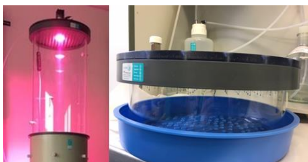
Fig. 2: Lighting and sprinkling unit.
