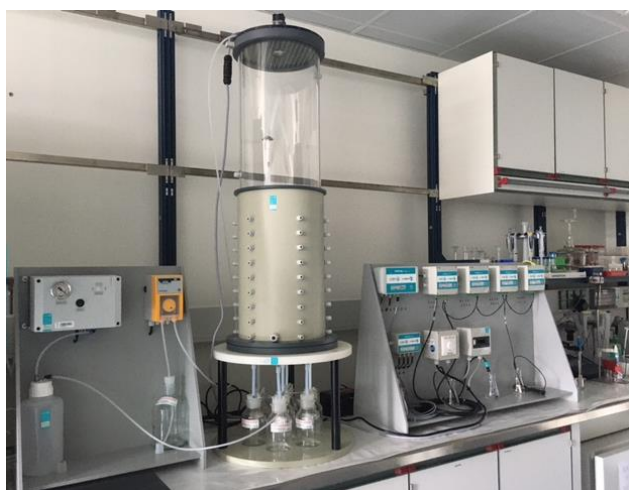
Fig. 1: Lab lysimeter system in the control area of the institute.
