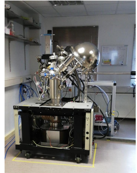
XPS facility in front of GaN chamber
