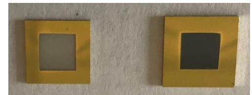
GaN on sapphire and Si sputtered with gold
