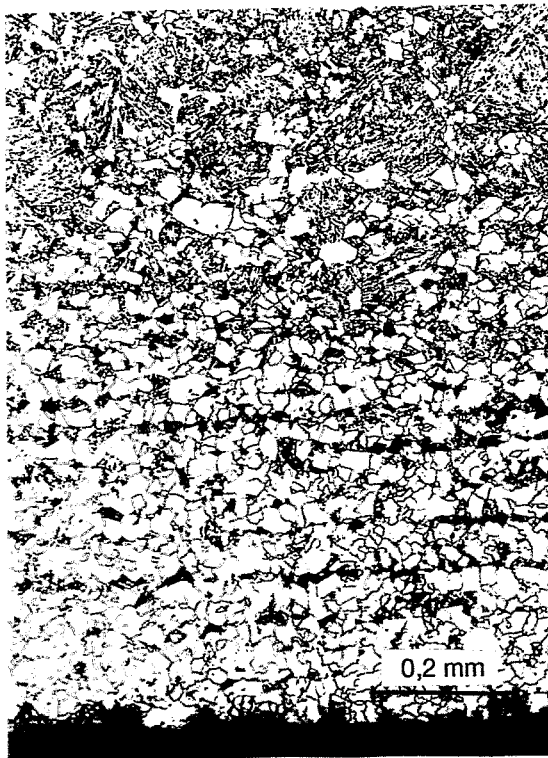
Fig. 27: Microstructure of sample C2/6, different locations over the wall thickness
