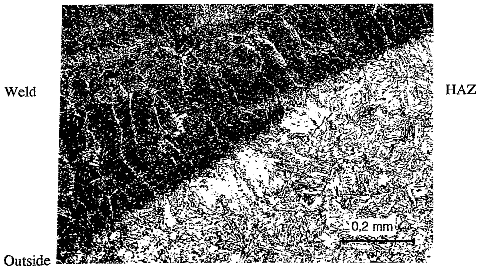
Fig. 9: Microstructure of sample C1/S, different locations over the wall thickness, weld and heat-affected zone (HAZ)
