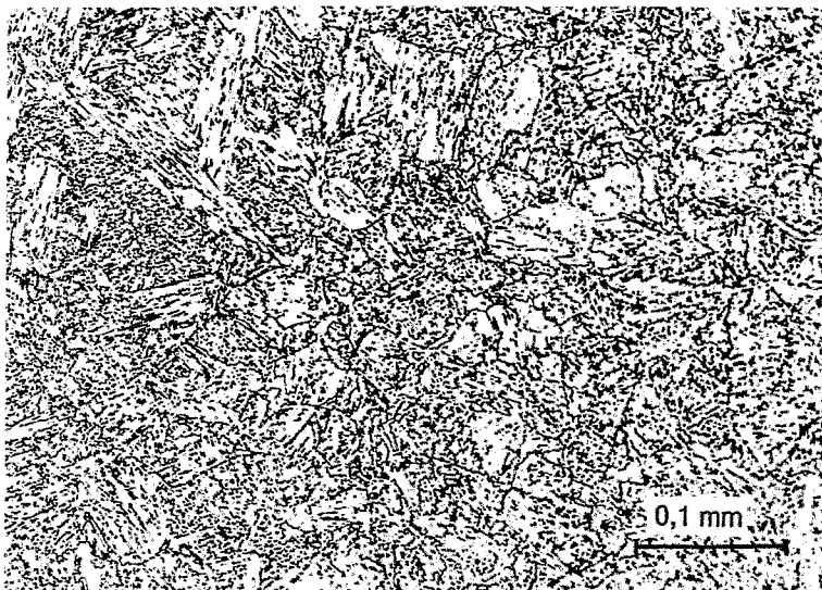
Fig. 44: Microstructure of sample C2/D, annealed: 1100°C/2 h, air cooling
