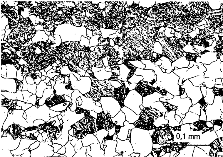
Fig. 43: Microstructure of sample C2/C, annealed: 1100°C/2 h, furnace cooling
