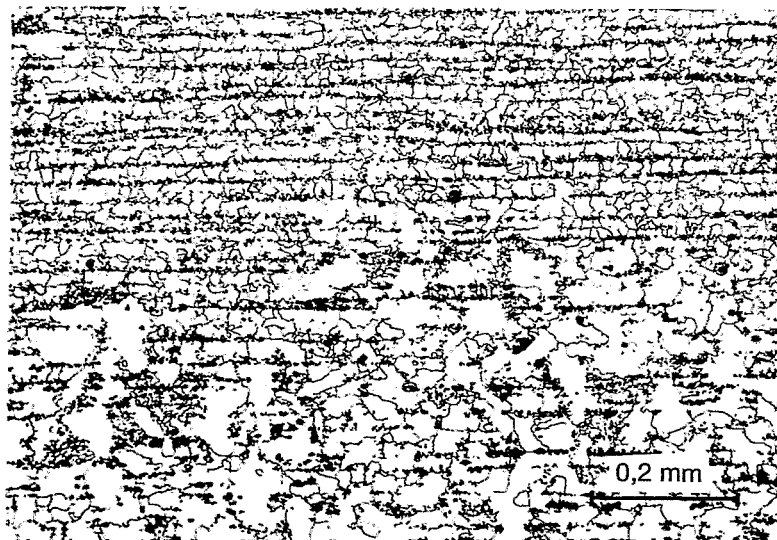
Fig. 13: Microstructure of sample C1/A, annealed: 700 °C/2 h, furnace cooling
