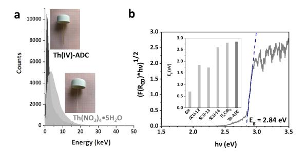
Figure 1. (a) The energy profile of particle detection of Th(IV)-ADC and Th(NO<sub>3</sub>)<sub>4</sub>•5H<sub>2</sub>O. The background count has been subtracted. The inset images are the respective capillaries loaded with pure samples; (b) The UV-Vis DRS of Th(IV)-ADC. The inset histogram is the comparison of the bandgap value of archetypical semiconducting materials for radiation detection.
