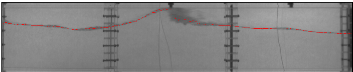
Fig. 9.2 Detected interface line (red) over original image from the high-speed camera during slug flow
