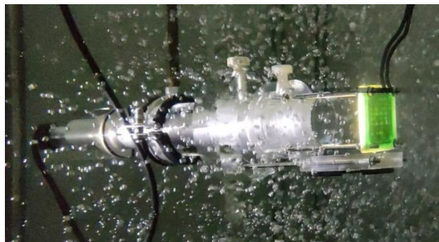
Figure 36 HZDR's in-situ flow microscope submerged in water experiencing bubbly flow.
