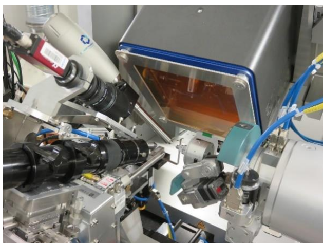
Figure 1. Experimental setup for electron density measurements at the XRD-2 diffractometer of the Rossendorf Beamline. [1] The Pilatus3X2M detector is tilted by 45 degrees.
