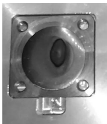
Figure 1. Opened target capsule after end of bombardment with the irradiated zirconium foil on top of the aluminum backing.
