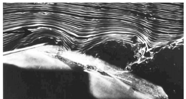
Fig. 2: Shear layer above a flap excited by an oscillating flaperon [9].
