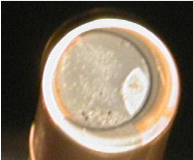
Fig. 2: Photograph of a gold-coated cathode with deposited Cs_2Te layer.
