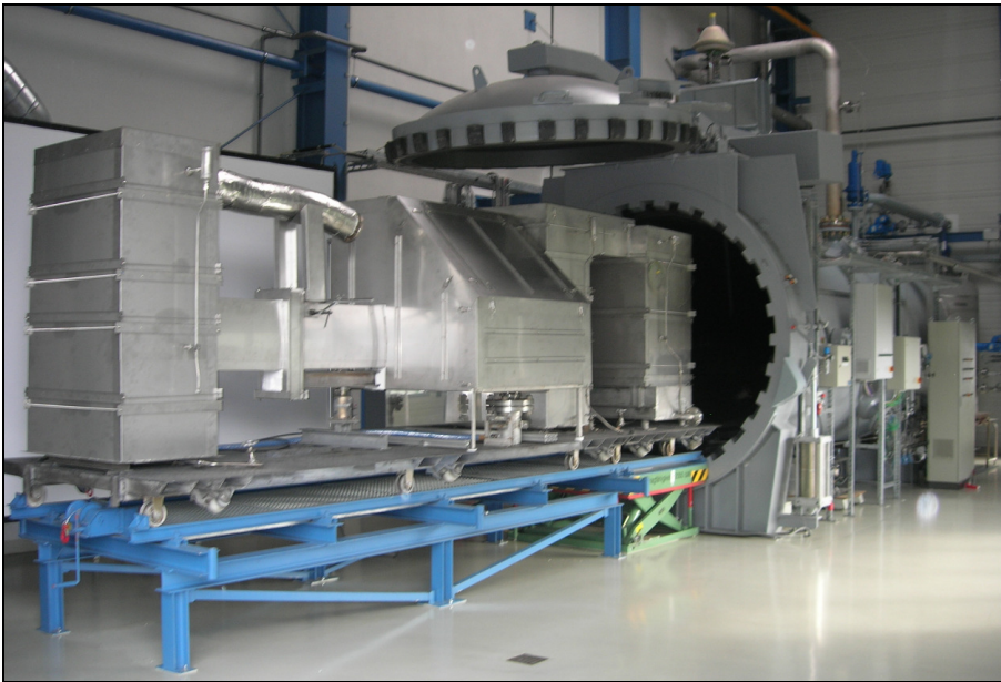
Fig. 2.7 insulated hot leg model test section
