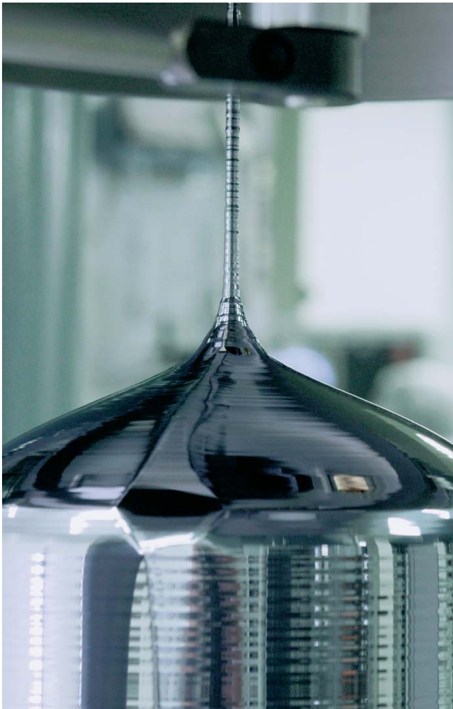
Fig. 1: A 300 mm silicon crystal grown by the Czochralski crystal growth process, picture by Siltronic AG.
