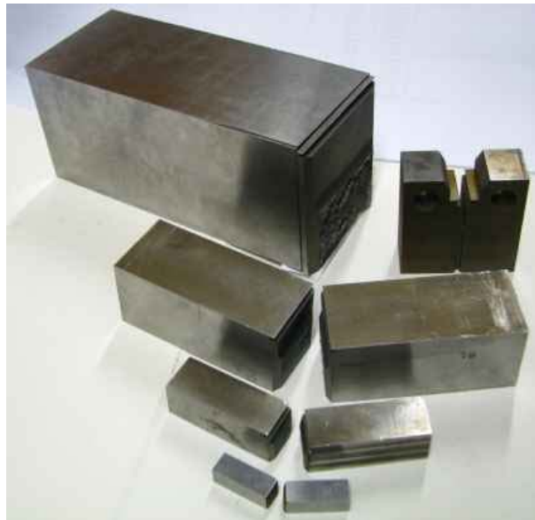
Fig. 3.1: Halves of the tested SE(B) specimens with B=0.4T , 0.8T , 1.6T and 3T as well as a 1T-C(T) specimen.
