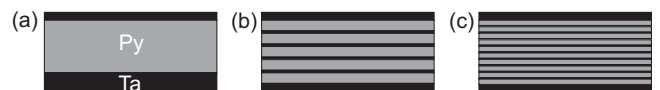
FIG. 1. Sketch of the Py/Ta thin film systems: (a) 1 \times \text{Py} , (b) 5 \times \text{Py} , and (c) 10 \times \text{Py} .
