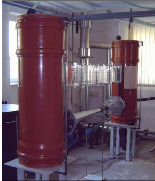
Figure 3.2: The horizontal channel for preliminary tests
