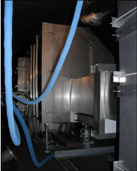
Figure 4.7: insulated test section mounted in the pressure chamber
