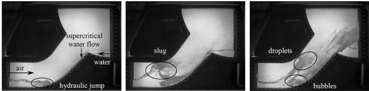
(a) \dot{m}_G = 0.345 \text{ kg/s} ; t = 21.50 \text{ s} (b) \dot{m}_G = 0.395 \text{ kg/s} ; t = 76.59 \text{ s} (c) \dot{m}_G = 0.41 \text{ kg/s} ; t = 97.92 \text{ s}
