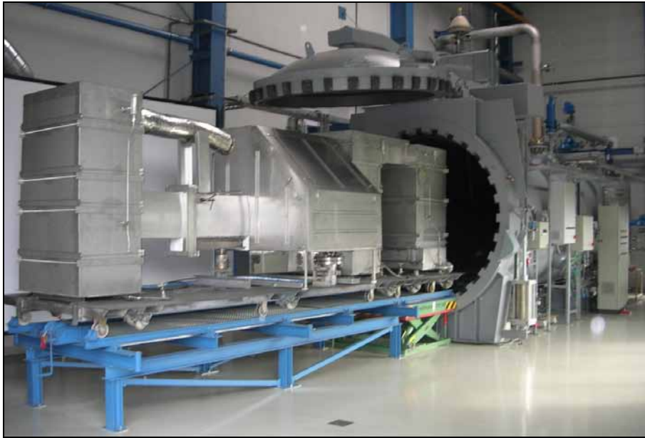
Figure 4.3: Complete experimental setup: the insulated hot leg test section in front of the pressure chamber of the TOPFLOW test facility
