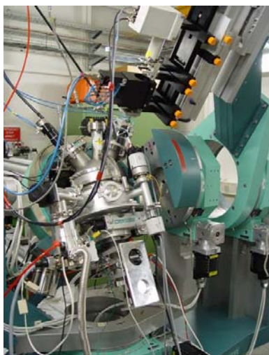
Fig. 1.: Sputter deposition chamber.
