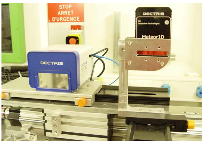
Fig. 1. Left, Pilatus 100K mounted on the detector bench. Right, Meteor 1D mounted dedicated holder.
