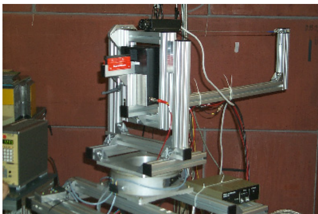
Fig. 1 The testing telescope for background studies. Two thin scintillators are fixed on a rotating step motor. A laser is used for position calibration.
