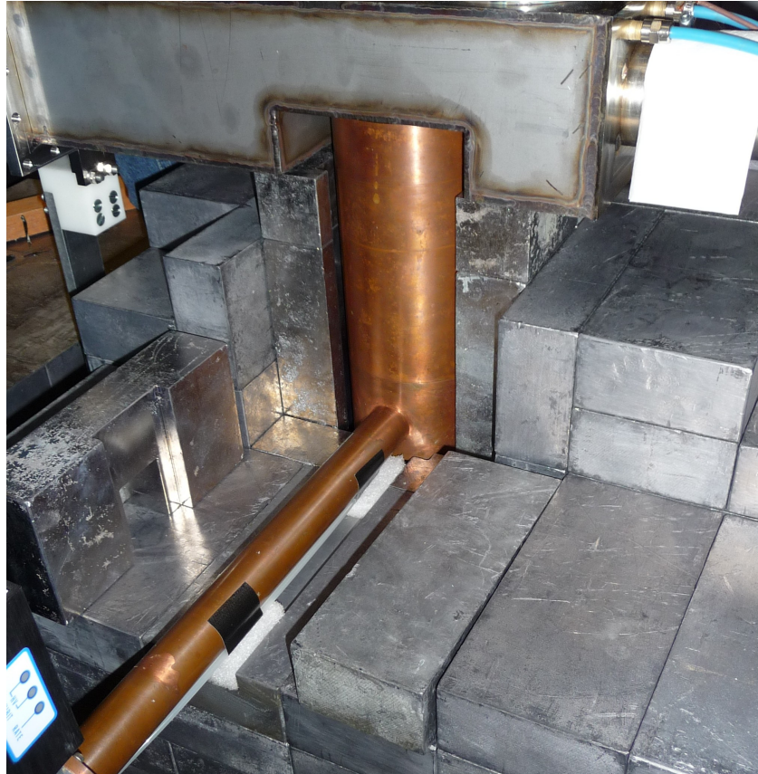
Figure 3.9.: The HPGe detector inside the surrounding lead shielding during construction. The small pipe below the cold finger conducted nitrogen gas inside the setup, to remove ^{222}\text{Rn} .
