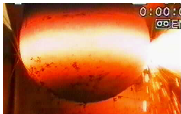
Figure 2-3: FOREVER-vessel at failure time
