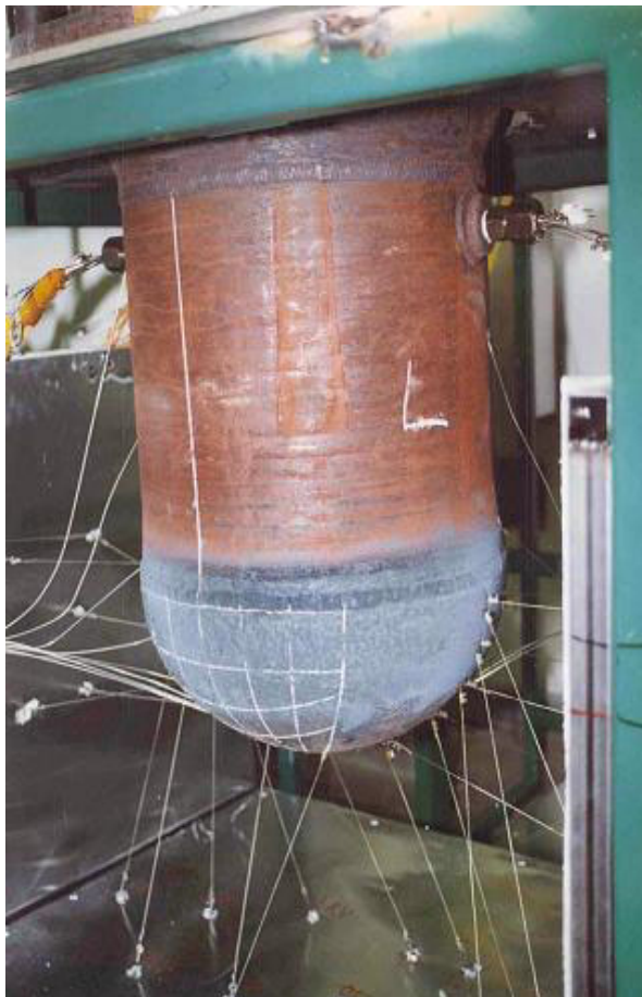
Figure 2-2: FOREVER-vessel with displacement sensors
