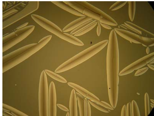
Fig. 1. Photo corresponding to about 3 x 2 mm 2 ZnO film surface area with partial defoliation from the SiC-6H substrate. ZnO film thickness was 1.3 µm.
