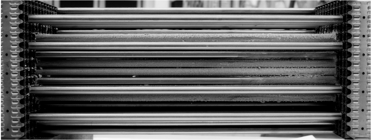
Figure 18: CP caused blockings inside the FA dummy (in dried state, after exp. no. ZFT-BE-V01; flow direction from left to right)
