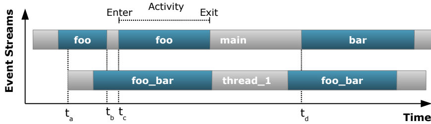
Fig. 1. Parallel event streams: An application trace with two parallel event streams. Each Enter and Exit event has a defined timestamp t . All events of an event stream are ordered by their temporal and semantic relations. Matching events form activities.
