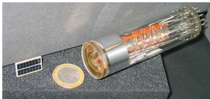
Figure 4.2: Photograph showing a 4 \times 8 pixels avalanche photodiode array (left), a 1 Euro coin (middle) and a photomultiplier tube with 1 inch front window (right).
