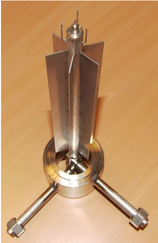
Figure 2.2: Gas injector M3 for small volume flows
